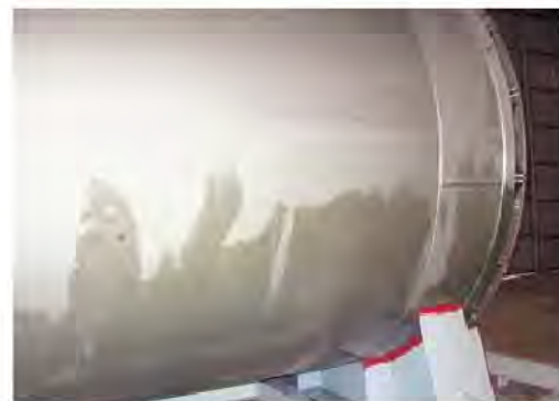
Avesta FinishOne™ Passivator 630- removes free iron (the brown staining seen on the photo).
